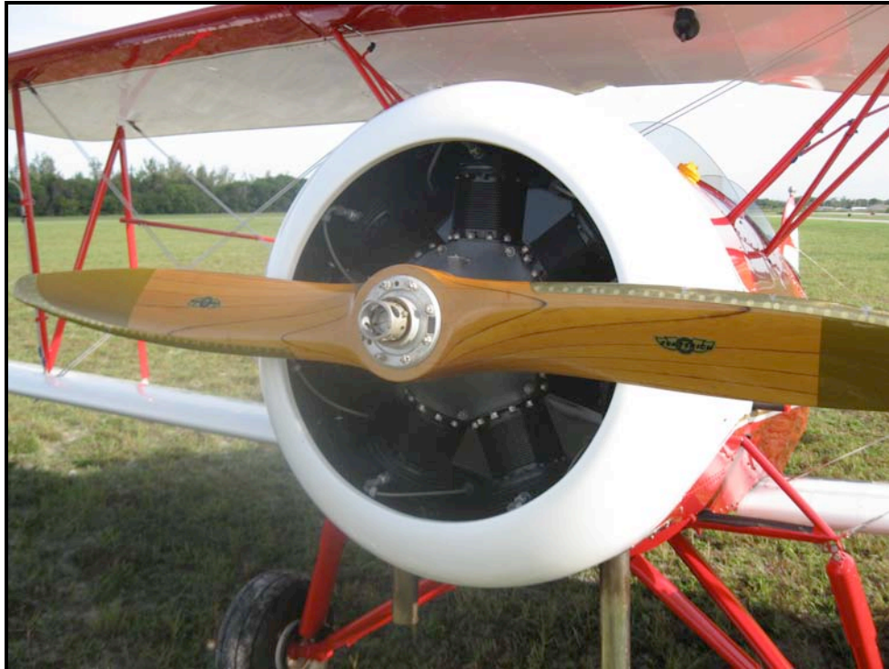
The New Sensenich Propeller With Warner Hub After Inspection And Cadmium Plating, and the rebuilt engine and cowling
