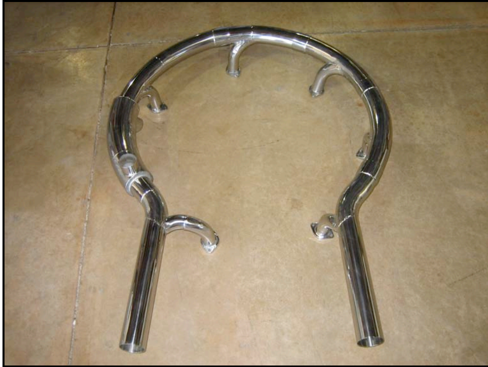
Photo of Engine Exhaust Collector
